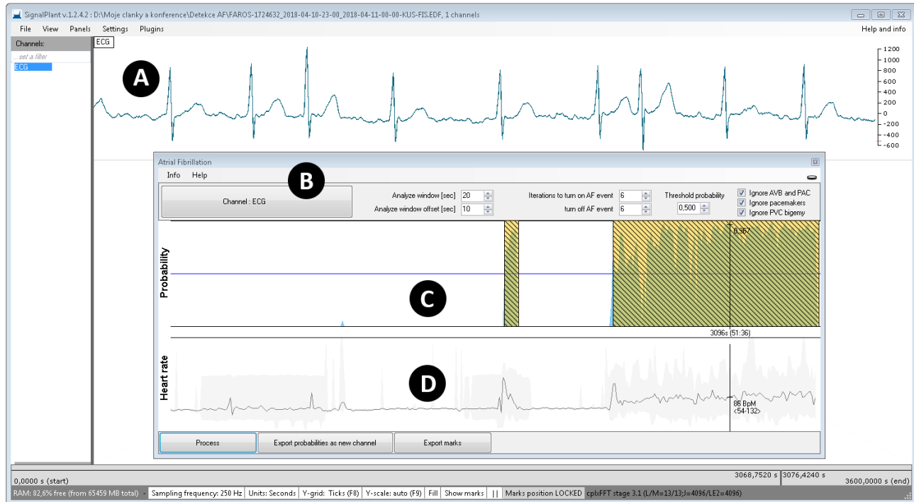
Figure 2. Software implementation of the presented model as a plugin for free SignalPlant [10] software (A). 1-hour ECG was loaded into SignalPlant; only 8 seconds of the signal is displayed. After processing, the plugin window (B) shows two panels: probability in time (C) and heart rate (D). The probability panel shows episodes of atrial fibrillation during the whole recording as hatched areas. The blue line is a threshold set at 0.5 by default; it can be changed. The heart rate panel (D) shows related BPM (median – black line, min/max – grey background). A click with the pointer in area (D) will show BPM values at a specific time and will also change the window displayed in (A); this allows the user to see the studied signal in detail.
