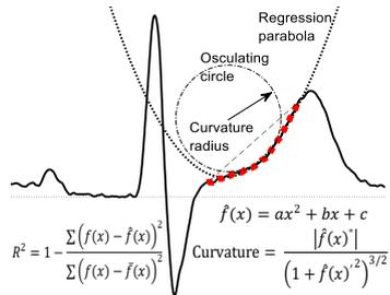
Figure 1. Example of quadratic polynomial regression of the ST-T segment and a curvature radius
