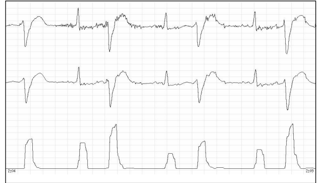
Fig. 4. Example of single channel ECG processing. From top to bottom: the original ECG, the low-pass filtered ECG, and the non-linearly scaled LT signal; 5 seconds per trace.
