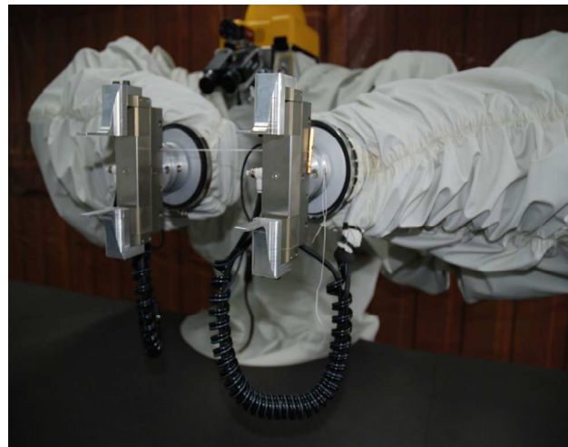
Figure 2. Two robot arms (Mitsubishi) with force sensors measuring the break force of each suture.
