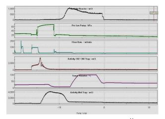
Figure 3. Graphical registration of the [<sup>11</sup>C]MHED synthesis parameters.
