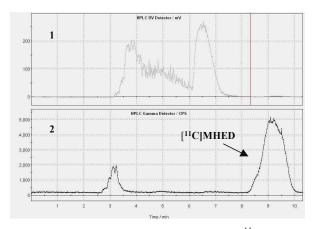
Figure 4. Semi preparative chromatogram of [<sup>11</sup>C]MHED purification: 1) UV/VIS trace, 2) Radiometric trace.
