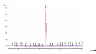
Figure 5. Analytical radiochromatogram of the final  $[^{11}C]MHED$  solution.
