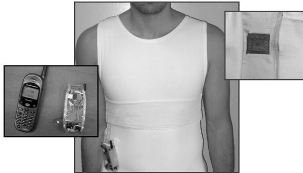
Figure 1. The MagIC system. As it can be seen the MagIC vest is very easy to be worn.
