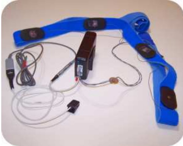
Figure 1: UPAD acquisition unit with ECG dry electrode belt and pulse oximeter.
