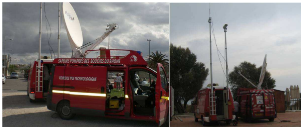
Figure 2. Emergency satellite-WiFi communication by SAFE.
