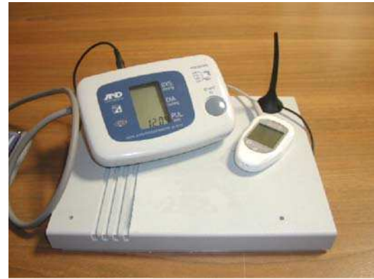
Figure 4. The Home Transmitting Unit, with the commercial blood pressure and blood glucose meters.
