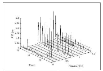
Figure 2. Typical example of *PSD* as a function of frequency, for different epochs, in a ZLR.
