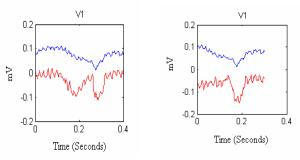
Figure 9. On the left, the extracted P wave signal (top) and the P wave on the T wave for patient 2. On the right, a comparison of the extracted P wave (top) to a separate reference P wave (bottom).
