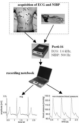
Figure 1: Measuring system for acquisition of ECG and non-invasive blood pressure.
