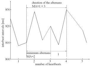
Figure 2: Determination of the alternans duration.
