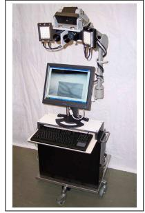
Figure 1. A trolley with the device consisting of 2 CMOS cameras plus 2 VIS/NIR LED-arrays on a swivelling arm, all connected to a dual Xeon processor PC.
