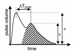
Fig 3 Depict the typical waveform of the DVP and its characteristic parameters as: time between the first and second tip ( $\Delta T_{DVP}$ ), amplitude of the first tip identified by (a), amplitude of the second tip identified by (b).
