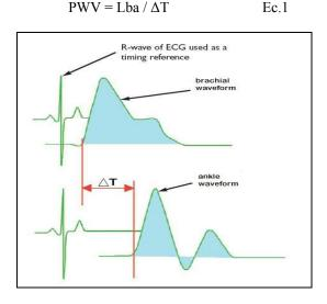
Figure 1 Example of signals detected by Doppler probe (brachial and ankle waveform) the R wave of ECG is used as timing reference to calculate  $\Delta T$ .
