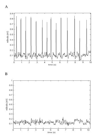
Figure 1. Ten-second ECG signal examples showing QRS wave reduction with ASVC. (A) Original 30-second ECG signal. (B) Resulting atrial signal after ASVC processing.
