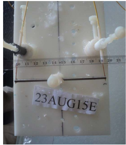
Figure 7. Set-up for thermal measurements of Ti rod
