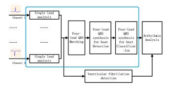
Figure 1. Schematic diagram of the four-lead real time arrhythmia analysis algorithm.
