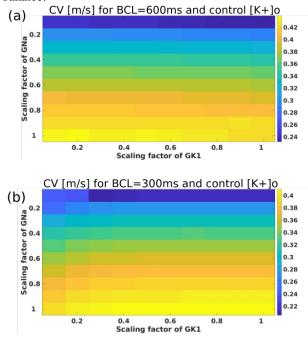
Figure 1. CV [m/s] along human 1D fibres for different scaling factors of the original conductances,  $G_{Na}$  and  $G_{K1}$ . (a) Low frequency pacing limit (BCL > 600 ms), where CV is solely governed by  $I_{Na}$  channel dynamics. (b) High frequency limit (BCL  $\leq$  300 ms), exhibiting a concomitant modulation of CV by both  $I_{Na}$  and  $I_{K1}$  currents.
