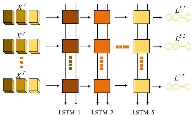
Figure 3: 5-layer LSTM network, in this figure, LSTM is a schematic diagram of the expansion along time.
