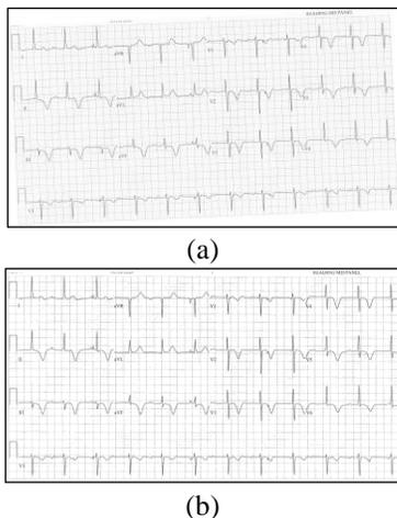
Figure 1. (a) Original skewed ECG image; (b) ECG image after skew correction.
