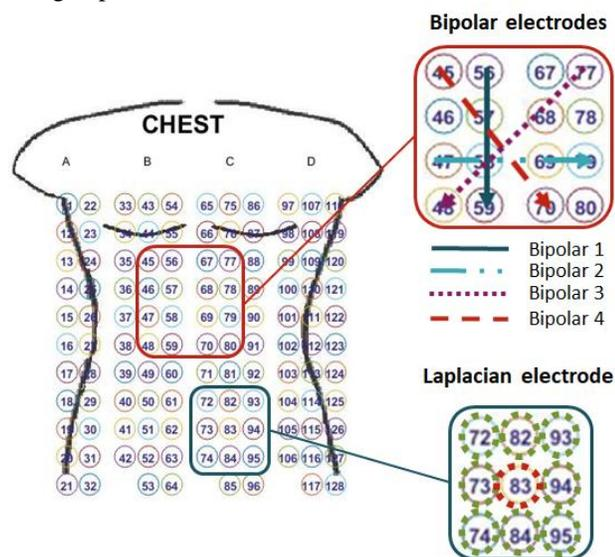
Figure 1: Chest electrode configuration. 72 Laplacian signals were created from the 128 body surface signals (bottom right) by subtracting the mean of the 8 neighbors (green dashed circle) from the central electrode signal (red dashed circle). Four bipolar signals were created (top right) in the 1. vertical, 2. horizontal, 3. right diagonal, 4. left diagonal directions.
