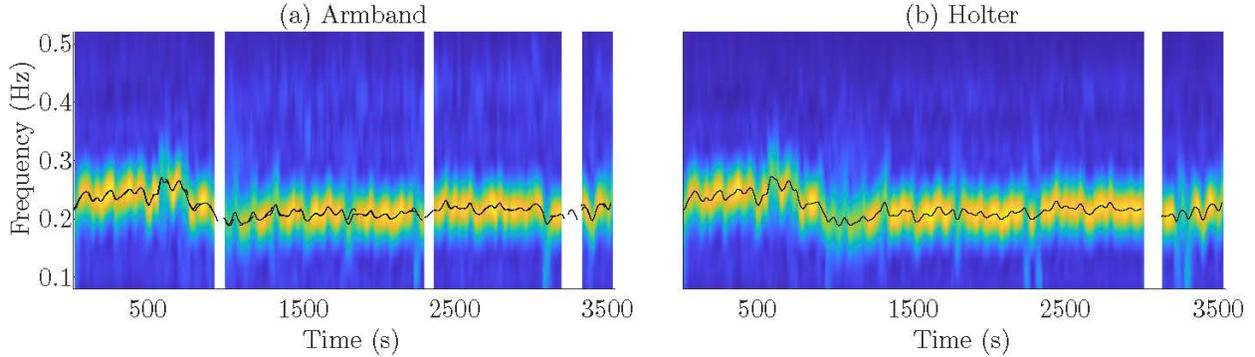
Figure 2. (a) Example of one hour of  $\bar{S}(k, f)$  obtained from the armband. The solid black line represents the estimated respiratory rate, and the slashed black line represents the reference (estimated from the Holter) respiratory rate. (b)  $\bar{S}(k, f)$  obtained from the Holter for the same subject during the same hour. The solid black line represents the reference respiratory rate. The white gaps represent those periods when the BR was not estimated.
