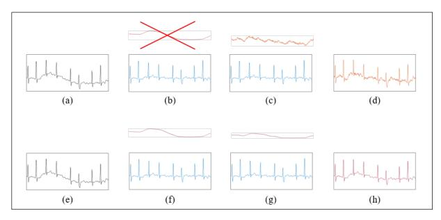
Figure 1. How the Recorded Noise (top) and Filtered Noise (bottom) datasets were generated. For the Recorded Noise dataset, (a) obtain raw data, (b) filter to obtain clean signal and noise, discard noise, (c) select segment of recorded noise and scale to specified SNR, (d) add recorded noise to the clean signal. For the Filtered Noise dataset, (e) obtain raw data, (f) filter to obtain clean signal and noise, (g) scale noise to specified SNR, (h) add scaled noise to the clean signal.
