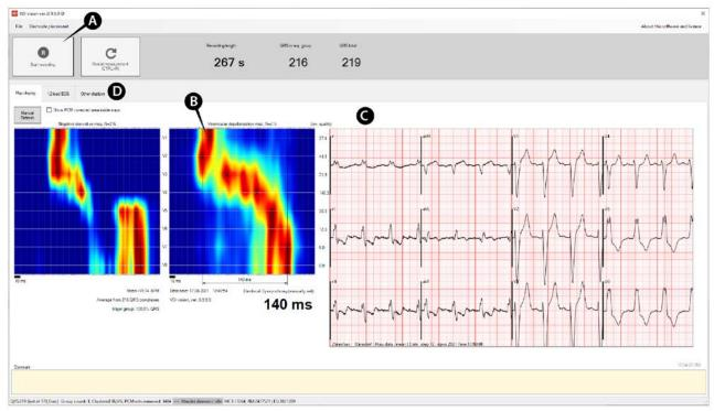
Fig. 1 – The VDI Vision software graphical unit interface when the measurement is finished. When a new measurement is started (A), the Ventricular Depolarization map (B) is instantly updated whenever a new QRS complex is detected in incoming ECG signal (C). Inner processes may be further checked using other display modes (D).
