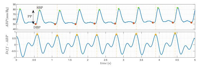
Figure 1. The top panel represents a 5 s segment of the ABP waveform. SBP and DBP, are indicated by green and red dots, respectively. The bottom panel shows the first difference of the ABP signal where yellow dots and dash lines show the peak value and instant of the first difference, respectively, associated to the time-stamp of the CBP.
