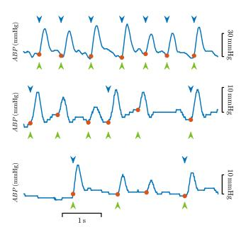
Figure 3. Three examples of the performance of the diastolic time-point detection algorithm. The gold standard annotations are shown as red dots, and the annotations of the algorithms in green (this study) and blue (wabp algorithm).
