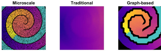
Figure 3. Graph-based homogenisation creates upscaled problems that respect the effects of intricate patterns of fibrotic obstruction (in black). Colours are as in Figure 1, with the stimulus located similarly. Traditional (volume averaged) homogenisation produces an upscaled model that faintly represents the spiral structure in its activation map, but obstacles are leaky and results wholly incorrect.
