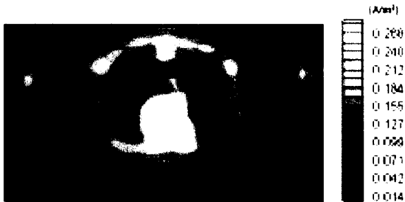
Fig.2 The distribution of the magnitude of the current density induced by trapezoidal waveform in the cross section including the heart.
