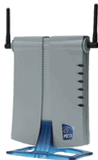
Figure 2: PicoBlue Bluetooth LAN Access Point
