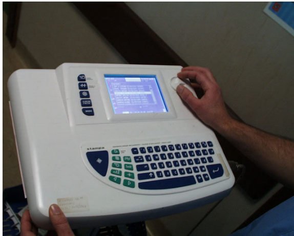
Figure 1. ECG device: the keyboard and screen allow patient name selection or, to insert a new patient name.
