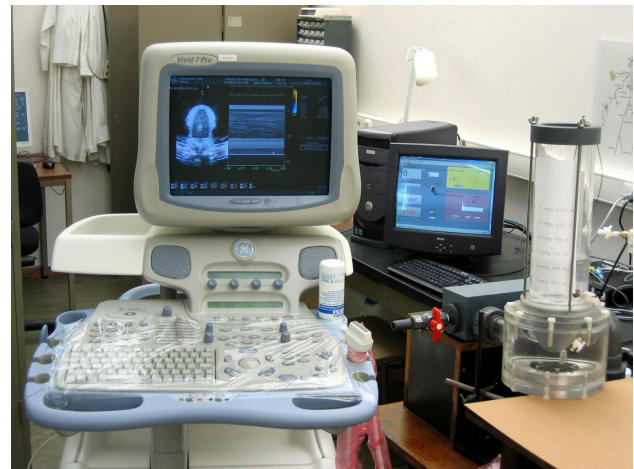
Figure 4: Experimental setup: Ultrasound scanner GE Vivid 7 Pro (left), computer controlled hydraulic model (right).
