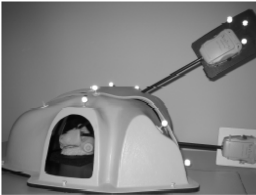
Fig. 6: „Patient“ (chest phantom) and instruments are equipped with infrared markers to allow tracking by an external camera system.
