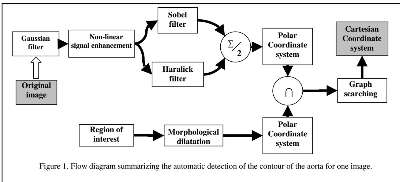
Figure 1. Flow diagram summarizing the automatic detection of the contour of the aorta for one image.
