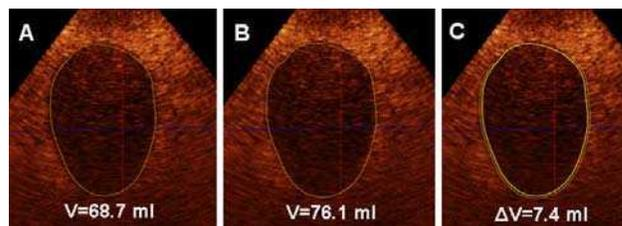
Figure 4. Long-axis cut-plane of the phantom extracted from a RT3DE dataset, shown with the boundary traced along the interface (A), after expanding the boundary 1 mm outwards (B) and with both boundaries (C). The small difference in boundary position resulted in an 11% difference in the measured volume.
