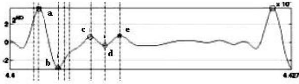
Figure 4. Systole and diastole waves of second derivative of PPG signal.
