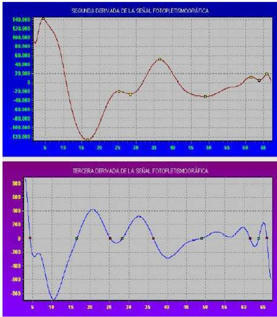
Figure 8. Second and third derivatives of PPG signal.
