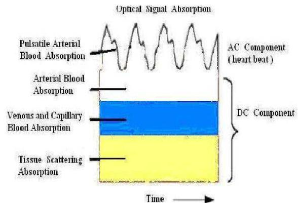
Figure 1 Variable and constant components of detected optical signal.
