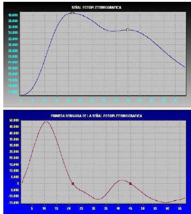
Figure 7. Original and first derivative of PPG signal.
