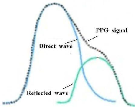
Figure 2. PPG signal and its component waves.
