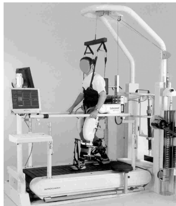
Figure 1. A participant ambulating on a treadmill with assistance from the Lokomat ( www.hocoma.ch )
