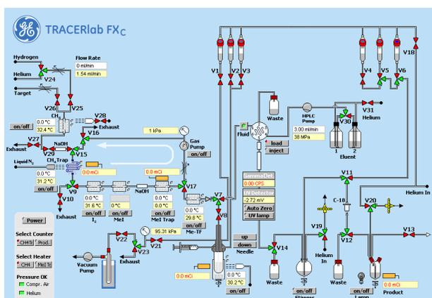
Figure 2. Graphical process panel of the module.
