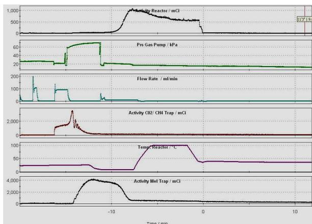
Figure 3. Graphical registration of the [ $^{11}\text{C}$ ]MHED synthesis parameters.
