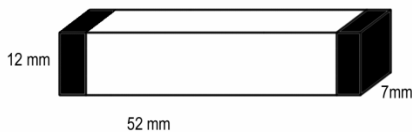
Figure 1. Horizontal illustration of the implant model. The insulated body in white and electrodes in black.
