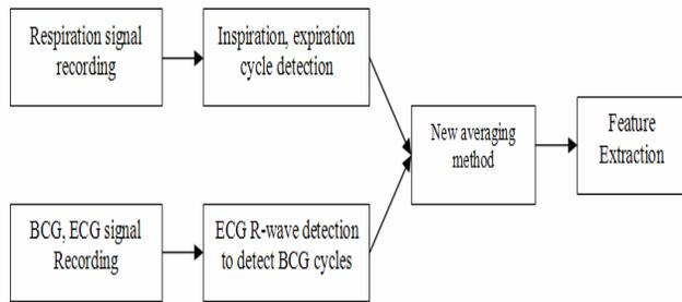
Figure 2. Our general BCG signal processing methodology using respiration information.
