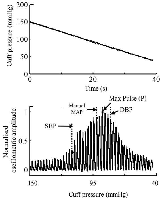
Figure 1. One typical example of cuff pressure (top) and extracted oscillometric pulse waveform (bottom).
