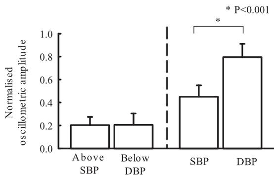
Figure 3. Paired comparisons of normalised oscillometric pulse amplitude between the pulses at cuff pressure above SBP and below DBP (left) and between the pulses associated with manual SBP and DBP (right).
