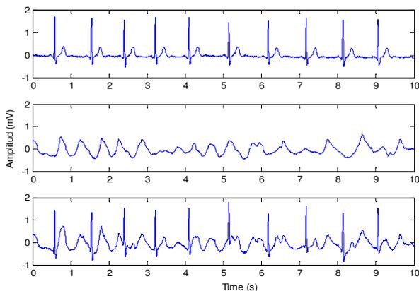
Figure 1. Extract of a clean ECG, a noise and the sum of both signals. The SNR of the combined signal is of 0 dB.
