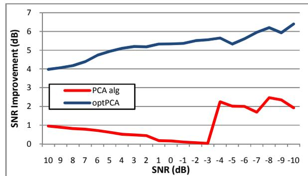
Figure 4. SNR improvement of PCA output and clean ECG signals plotted against SNR value when the selected PC were retained (PCA alg) and the optimal subset of principal components were retained (optPCA).
