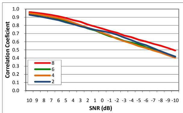
Figure 5. Correlation Coefficient of PCA output and clean ECG signals plotted against SNR value for different number of input signals. The optimal principal component for each signal and SNR was retained.
