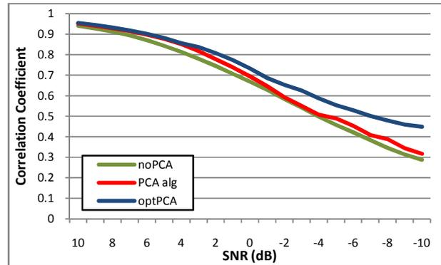
Figure 3. Correlation coefficient of PCA output and clean ECG signals plotted against SNR value when the selected PC were retained (PCA alg), the optimal subset of principal components were retained (optPCA) and the median correlation coefficient of noisy ECG with clean ECG signals (noPCA).
