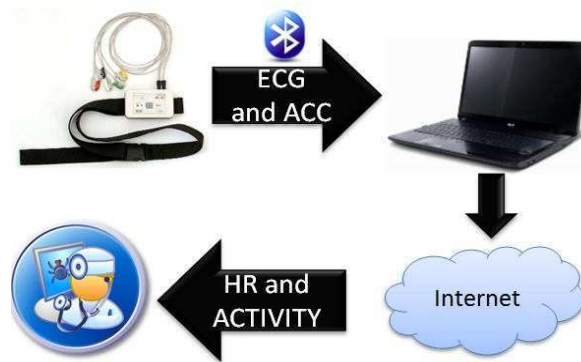
Figure 1. Data flow in wireless monitoring system.
