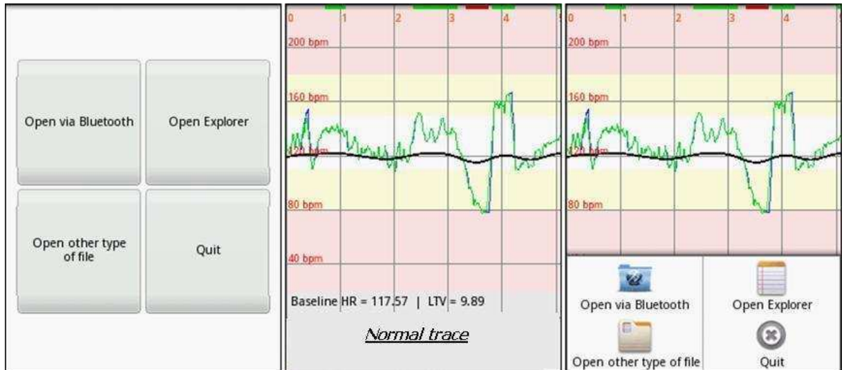
Figure 4. Graphical user interface and visualization of the signal together with the indication of FIGO rules fulfillment
