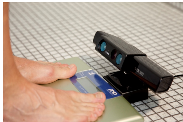
Figure 2. Illustration of the sensor system, consisting of a 3D camera in combination with a body weight scales.
