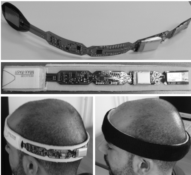
Figure 1. Some snapshots of the developed wearable device. The figure shows the flexible kapton PCB embedding the Nellcor Max-Fast forehead reflectance sensor, the insertion of the PCB in the Nellcor Max-Fast headband, and the easy way to wear the system.
