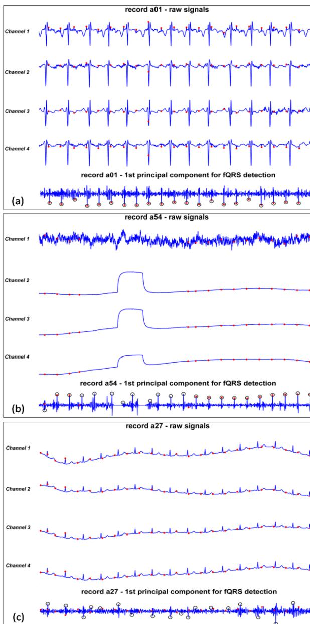
Figure 3. Example of good signal and good algorithm performance (a); noisy signal and good algorithm performance (b); good signal but with poor algorithm performance (c). Red dots are the reference fR-peaks; black circles are the ones computed by this algorithm.
