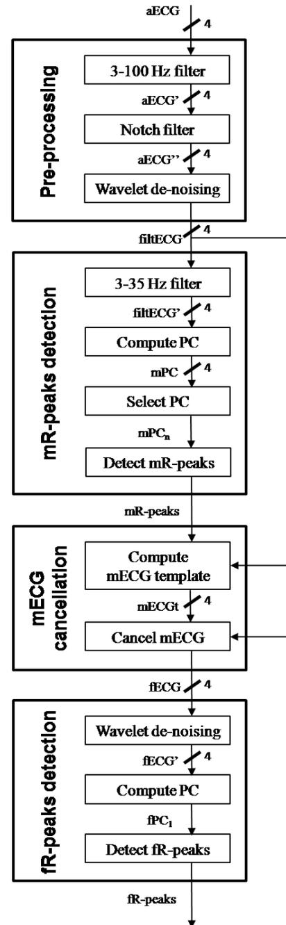
Figure 2. Diagram describing the algorithm.
