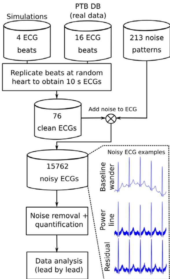
Figure 1. Flowchart illustrating noisy ECG.s creation and signal processing.
