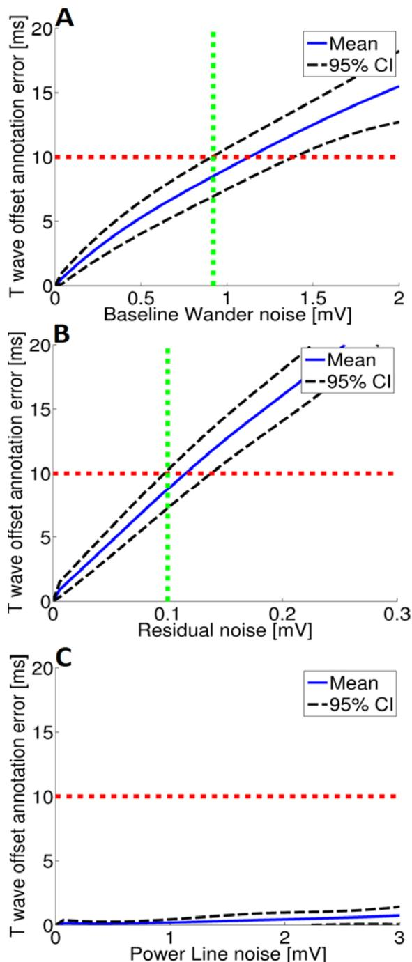
Figure 2. Mean and 95%CI of T offset annotation error vs. baseline wander (A), residual (B) and power-line (C) noise. The horizontal dotted lines represent 10 ms arbitrary noise limit and the vertical dotted lines mark its intersection with the upper 95% confidence interval. Plot limits were chosen to show ranges of interest.
