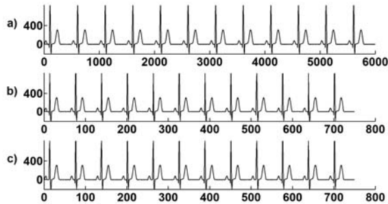
Figure 6. ANE20000 with small HF noise. N=8 . a – input, b – new algorithm output, c – original algorithm output
