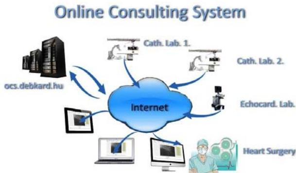
Figure 1. The communicates via Internet by VPN connections among the DICOM servers of the catheterization laboratories.
