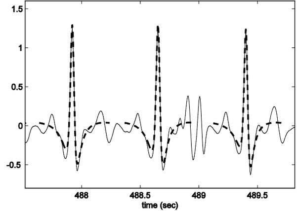
Figure 5. Rational approximation of QRS complexes. The dashed curves are graphs of Malmquist-Takenaka partial sums.
