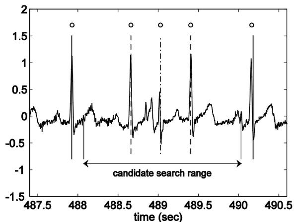
Figure 3. Overview of the rhythm-based algorithm. The dash-dotted location in the middle is being skipped and replaced by the dashed candidates found in the candidate search range. All subsets of the candidates in the search range are examined, and the ones with lowest score are selected. Since the dashed locations are more in-rhythm, the algorithm chooses them instead of the dash-dotted location. The small circles mark the location of the candidates.
