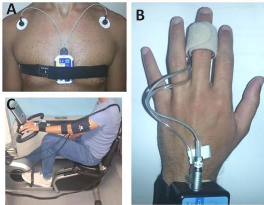
Figure 2. Instrumentation used for the study. *Panel A:* the MagIC-SGC placed on the subject's thorax. *Panel B:* detail of the finger cuff used to detect BP. *Panel C:* detail of the subject on the cycloergometer
