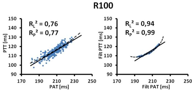
Fig. 5 PTT vs. PAT scatter plots before (*left panel*) and after (*right panel*) filtering. Data refers to subject 5 at R100.  $R_L^2$  and  $R_p^2$  are the coefficients of determination computed by linear and parabolic regression analysis, respectively.
